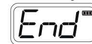
It indicates end of unit life, and the product needs to be replaced.
